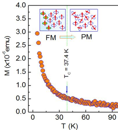
**Fig. 5:** The temperature dependence of magnetization for ZnO nanowires doped with 0.12 at.% Mn
