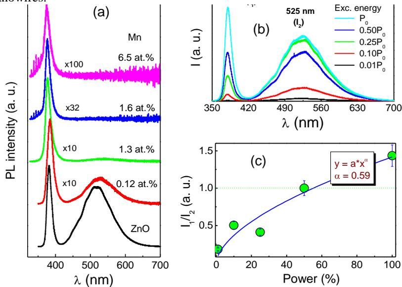
**Fig. 3:** (a) PL spectra of pure and Mn-doped ZnO nanowires under an excitation line of 325 nm; (b) PL spectra of the 0.12 at.% Mn sample under different excitation powers; (c) the power dependence of the  $I_1/I_2$  ratio fits to a function of  $y = ax^\alpha$
