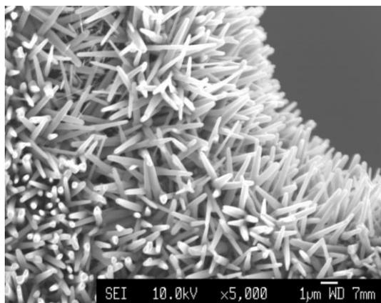
*Fig. 1: A representative FE-SEM for ZnO nanowires doped with Mn*
