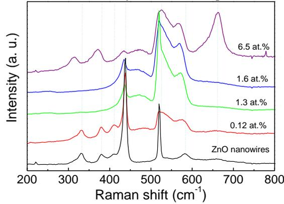
**Fig. 4:** Raman scattering spectra for ZnO nanowires doped with Mn
