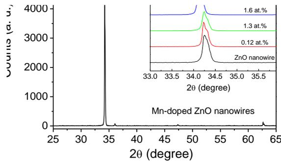
**Fig. 2:** X-ray diffraction patterns for ZnO nanowires doped with Mn at different concentrations
